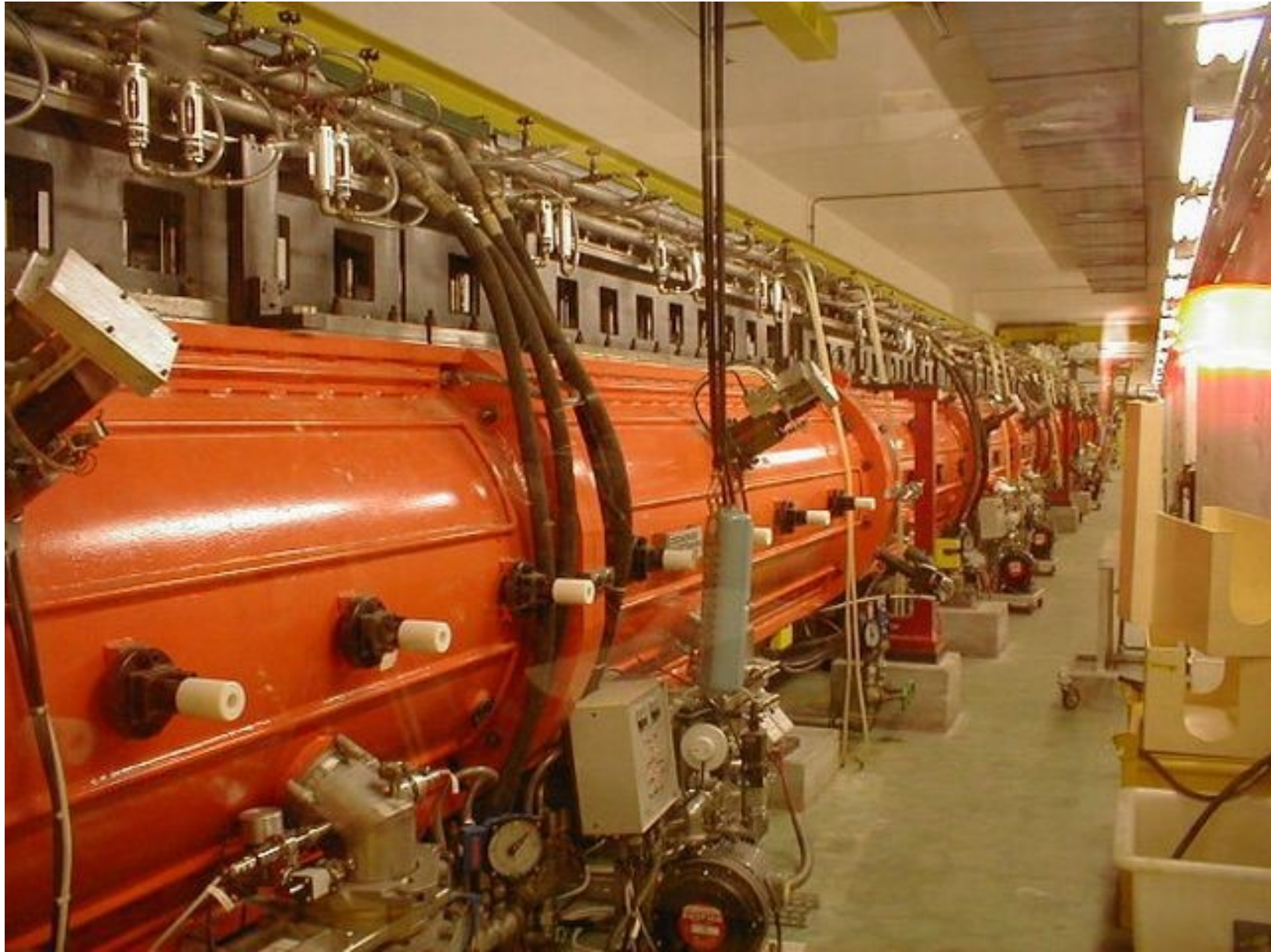
CERN Linac2 (protons, 50 MeV)
